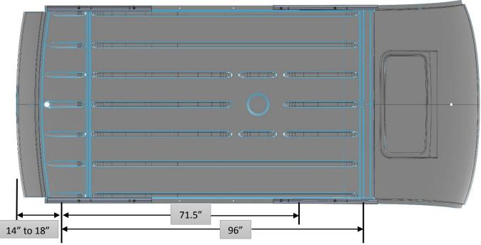
Nextremove the plugs from the roof in the desired location and bolt rails foam side down using M8x40mm BHCS(x) and flat washers (n), with rubber washer(u), fender washer(y) and M8 nyloc nut (w) on the inside, as shown. Repeat until all the rail are in place, driver side should be a mirror of the passenger side. USE E6000 AROUND HOLES TO PREVENT LEAKS.
