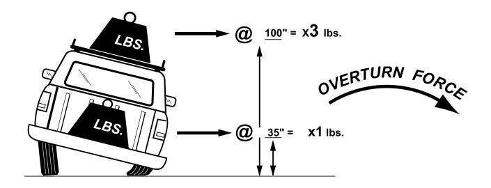
WEIGHT CARRIED ABOVE THE FLOOR OF THE TRUCK BED (E.G. ON AN OVERHEAD TRUCK RACK) WILL SIGNIFICANTLY INCREASE THE VEHICLE'S TENDENCY TO OVERTURN. ALWAYS KEEP HEAVY LOADS EVENLY DISTRIBUTED AND AS LOW AS POSSIBLE. IT IS IMPORTANT TO NOTE THAT THE KARGO MASTER RACK LOAD BEARING CAPACITY MAY BE GREATER THAN YOUR TRUCK'S GAWR OR GVWR CAPACITY, AND IS PROBABLY GREATER THAN THE WEIGHT THAT CAN BE SAFELY CARRIED OVERHEAD.
