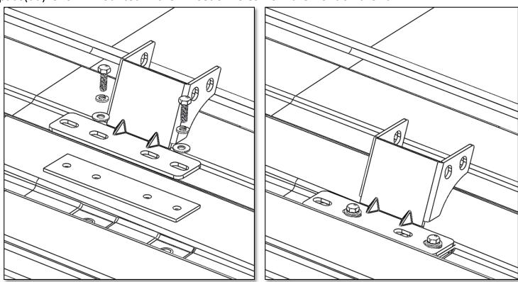
Locate <u>rear mounting bosses</u> on your Metris, remove plugs. Attach the mounting feet 80080-10-011 using 2 M6x20mm bolts(aa) with lock washers(bb), flat washers(cc) and rubber pads(dd). Feet should be vertical when done. Then place assembled ladder rack onto roof of van. Have the tapered sides facing towards the front to the van.
