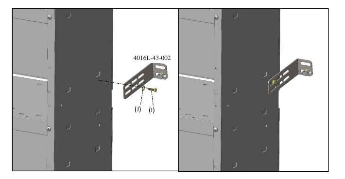
Attach 4016L-43-003 (bracket) to the opposite side of the shelf through the bottom slot using one <sup>1</sup>/<sub>4</sub>" x 7/8" bolt (I), two <sup>1</sup>/<sub>4</sub>" flat washers(J), one <sup>1</sup>/<sub>4</sub>"Nyloc nut(K)in the order shown below. HAND TIGHTEN ONLY
