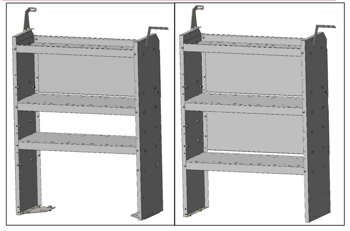
**Option 1**: Bottom Shelf up 1 location, lower "Back Panel" removed. "4016L-43-001" plates mounted to the bottom of the shelf allowing the shelf to be offset from the "D" rings. Allows shelf to be moved closer to the wall giving more aisle room. **Option 2**: Bottom Shelf on bottom location, lower "Back Panel" in place. 4832L mounts directly to "D" rings. Allows Kargo Master Drawer units to be mounted to the bottom shelf.
