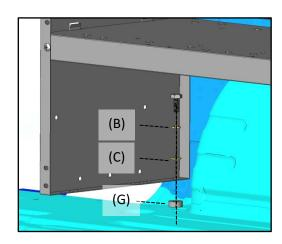
• Bolt 4016L-43-006 (7) to the upper rear weldnut using a M8 hex head bolt (O), one lock washer (U) and one flat washer (E). Bolt 4016A-43-006 (7) to the shelf using <sup>1</sup>/<sub>4</sub>" hex head bolt (I), with two flat washers (J), and one <sup>1</sup>/<sub>4</sub>" nylock nut (K)
