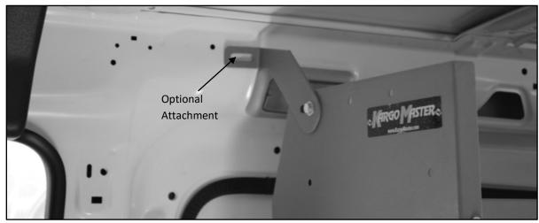
The "4016L-43-003" is used on the front side of the shelf and mounted to the factory M8 stud on the wall of the van, as shown below.
