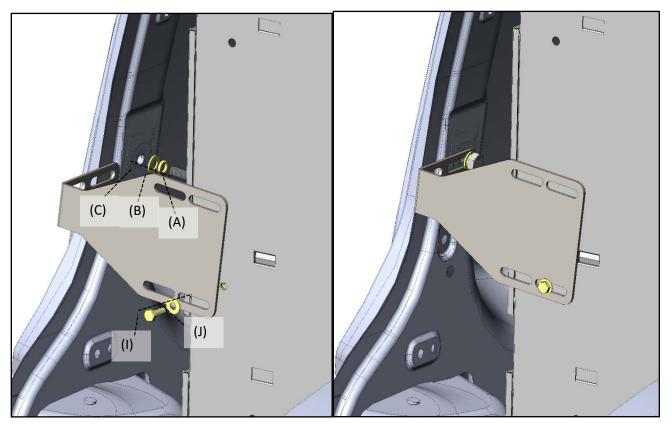
**Step 10** Level and align shelf. Finish by tightening all nuts and bolts.
