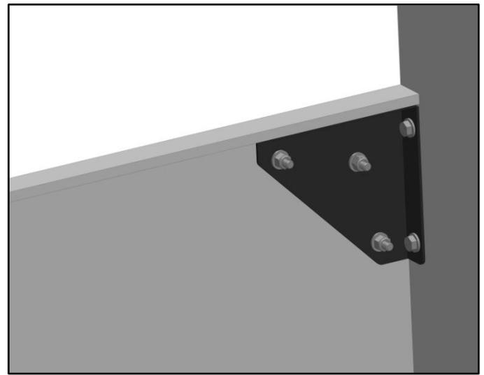
We recommend installing support tube (11-00757) to the front legs directly behind the cab of the vehicle. If front legs already bolted to top assembly, replace 1/2" x 2.5" Button head bolt with a 1/2" x 3.25" bolt. Along with bolt, use two 1/2" flat washers and a 1/2" Nyloc Nut.
