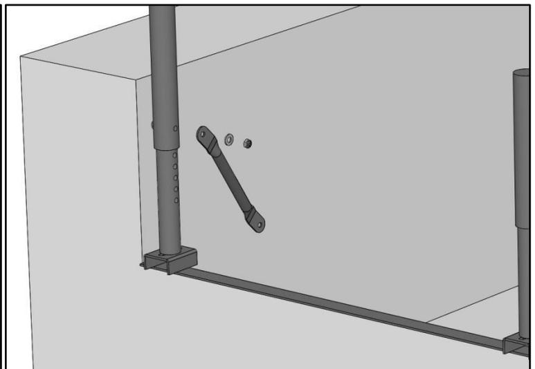
Approximately align your tube at a 45 degree angle. Mark through the bottom hole of the support tube into the side of your service body.
