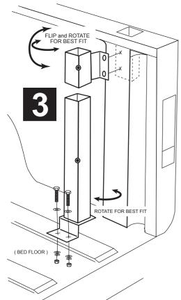
STEP 3 - The rear upright bracket will be bolted to the vertical face (inside face or forward face) of the inner bed wall around the rear stake pocket. With the rear upright inserted and plumb, locate the bracket flange so that the holes are at the approximate center of the stake pocket, as high as possible so that the bolt ends and nuts will be accessible. Mark and drill the inner bed wall at the stake pocket.
