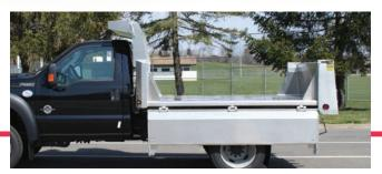
Fold down sides feature a centrally located quick release lever that extends and retracts <sup>3</sup>/<sub>4</sub>" pins at each end using a solid linkage member. Weight-saving aluminum fold down sides are optional on steel bodies.
