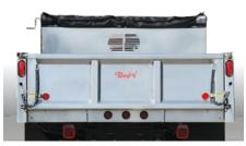
6° slope tailgate allows easy attachment of spreaders during winter.
