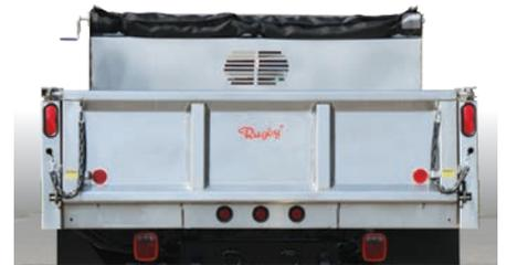
6° slope tailgate allows easy attachment of spreaders during winter.
