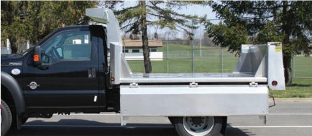
Fold down sides feature a centrally located quick release lever that extends and retracts 3/4" pins at each end using a solid linkage member. Weight-saving aluminum fold down sides are optional on steel bodies.
