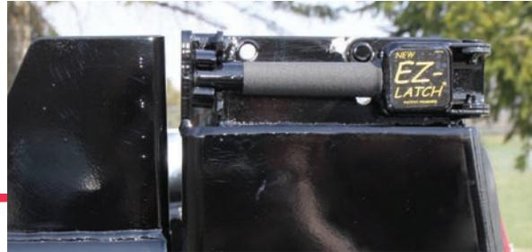
Rugby's patented and industry leading EZ-LATCH™ (located on each side of body) allows for easy body access. The latch system is designed for quick opening and slam lock operation with a cam action to draw-in upper tailgate pins.
