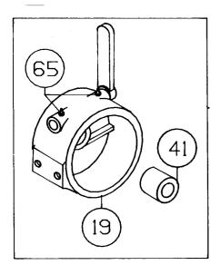
11. Check clutch housing bushing (item #4[) for wear. If necessary, remove old bushing and press new bushing into place. Apply grease to lube fittings (item #65) to lubricate clutch shifter shaft.
