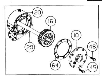
13. Apply grease to end of shaft, opposite gear. Apply grease to bushing in gear housing (item #20). Place greased end of shaft through bushing in gear housing (item #20). Place gasket (item #64) onto gear housing cover (item #10). Apply grease to gear end of shaft and cover bushing. Place cover onto shaft and secure to housing with seven (item #46) and one (item #45) capscrews. Tighten capscrews to 12 ft. lbs. (16.1 Nm.) each.
