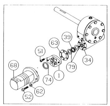
SAFETY BRAKE. Remove brake housing (item #18) from gear housing by unscrewing six (item #52) capscrews. Remove worm (item #35) and bearings (item #40) from gear housing. Use a soft hammer to gently tap input end of worm and drive worm and bearing from gear housing. Once worm has been removed from housing, bearing can be pressed from end of worm.
