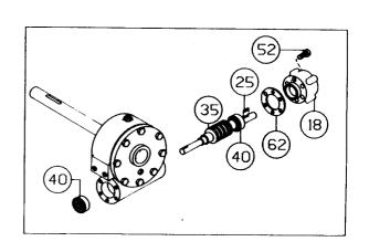
15. Press bearing (item #40) onto worm and into gear housing. NOTE: Be sure that thick shoulder of bearings outer race (side with manufacturer's name and part number) is out, away from worm threads. Attach bearing cap (item #8), to gear housing. Use six (item #44) capscrews to secure. Tighten capscrews to 18 ft. lbs. (24.4 Nm.) each. Tap key (item #25) into keyway.
