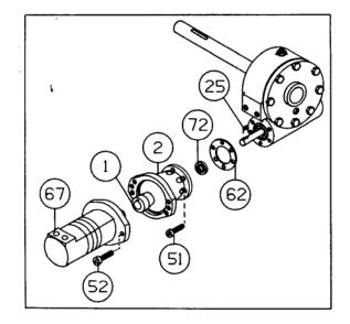
4a. Remove motor (item #68) from adapter (item #1) by removing two capscrews and lockwashers (items #52 & #62). Remove adapter (item #1) from gear housing by removing six (item #51) capscrews. Replace seal (item #74) and gasket (item #63). Remove thrust bearing (item #39) and thrust washer (item #79).
