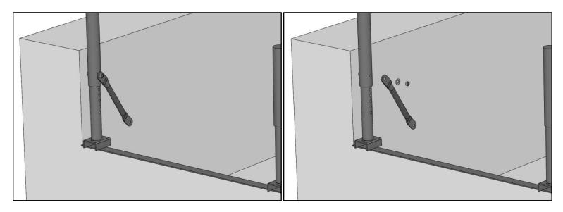
Approximately align your tube at a 45 degree angle. Mark through the bottom hole of the support tube into the side of your service body.
