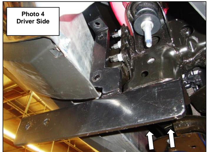
**Step-5** Position and attach (1) auxiliary bracket to the driver side lower bracket extension using (2) ½" x 4 ½" hex bolts, (2) ½" flat washers, (2) ½" lock washers and (2) ½" hex nuts, **(Photo 5 & 6)**. Leave the bolts loose for final adjustment.
