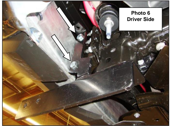
**Step-6** From the front of the vehicle, insert the driver side upper bracket through the opening in the bumper valance, **(Photo 7)**.
