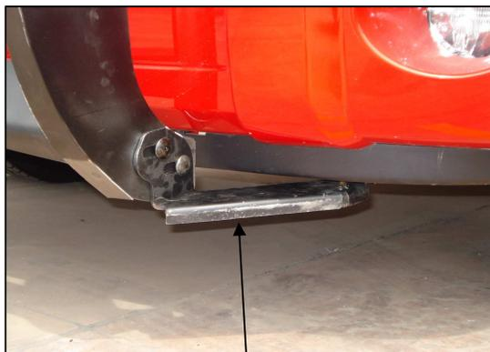
Bracket principal instalado, lado conductor.
