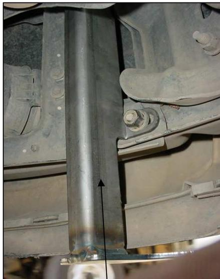
Bracket principal instalado, lado conductor.
