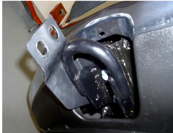
6. If the vehicle does not have tow hooks, use the template, (printed at the end) as a guide to modify the lower valance. **NOTE:** Before proceeding with the valance modification, make sure that the supplied paper template has the dimensions clearly printed and check them out. **PROFESSIONAL INSTALLATION RECOMMENDED.**
