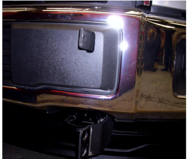
12 . Place Front grille guard as **Photo 7**, to secure lower bracket use 1/2 x 1 1/2" hex bolt, 1/2" flat washer and 1/2" lock nut. Secure to auxiliary bracket using 3/8 x 1 1/4" hex bolt, 3/8" flat washer and 3/8" lock nut. Leave loose.
