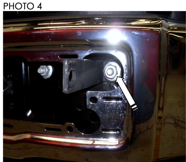
11. After installing the auxiliary bracket cut the plastic front part of the. Bumper valance tho allow the proper position. Tighten the nut befor puting the bumper valance back. Photo 5 and 6
