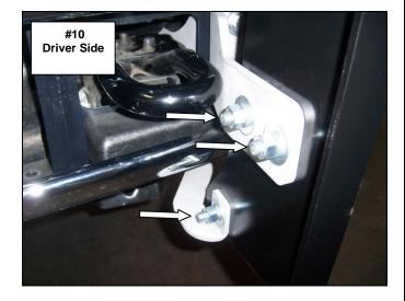
**Step -10** Level and adjust the grille guard and bumper, (if necessary), and tighten all nuts and bolts at this time.
