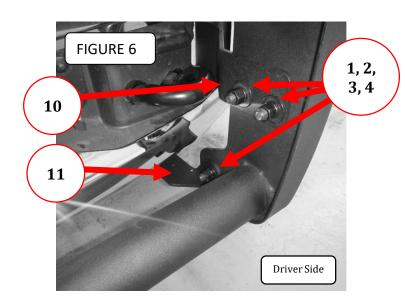
**Step-6** Align the Wrangler Guard with the front of vehicle and tighten all OEM and supplied nuts and bolts. Remember to check and retighten all nus and bolts periodically.
