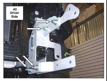
**Step-3** Remove the nuts (4) per side, the bumper brackets and the inner bolts (2) per side from the front bumper. Retain the nuts to reattach the front bumper; the bumper brackets will not be reinstalled. **Picture #3**
