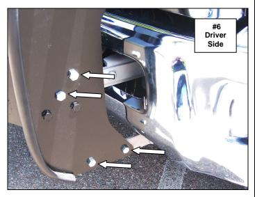
**Step-8** Position the driver side brush guard up to the grille guard side plate, align the holes and secure the bottom of the brush guard to the side plate using (1) 3/8" x 1 1/4" hex bolt and (1) 3/8" lock washer. Align the holes and secure the top of the brush guard to the side plate using (2) 3/8" x 1 1/4" hex bolts, (2) 3/8" flat washers and (2) 3/8" lock nuts. **Picture #7**
