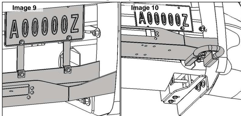
**13-** To reinstall tow hooks place them underneath the winch tray, using (2) 1/2 x 1 1/4" hex head bolts, (2) 1/2" flat washers and (2) 1/2" lock nuts, for each tow hook. Use black plated hardware. Image 10.
