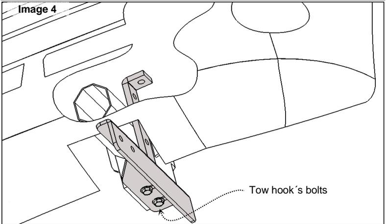
9- Auxiliary bracket complement lower bracket, see image 5 to install. Use (2) 1/2 x 4 1/2" hex head bolt, (4) 1/2" flat washers, (2) 1/2" lock washers and (2) 1/2" hex nuts. Repeat for the opposite side.
