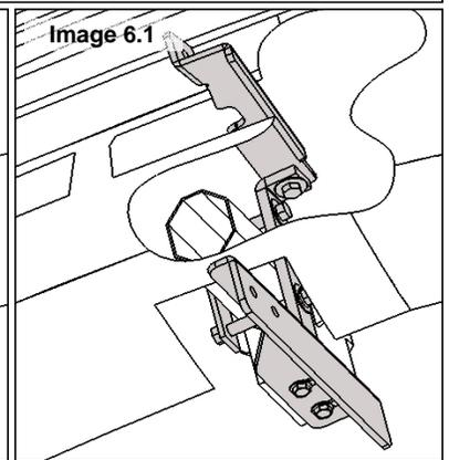
**11. ATTENTION!! Image 7 for models 2007 to 2009 and image 7.1 for models 2010.** Secure lower brackets to Grille Guard with (2) 1/2 x 1 1/4" hex head bolts, (2) 1/2" flat washers and (2) 1/2" lock nuts. Attach top bracket with (1) 1/2 x 1 1/4" hex head bolts, (2) 1/2" flat washers, (1) 1/2" lock nut. All hardware is black plated.
