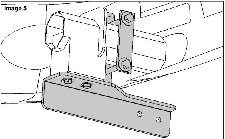
10- **ATTENTION!!** Installation of top brackets varies according model. For models 2007 to 2009 see image 6 and for models 2010 see image 6.1. Use (1) 1/2 x 1 1/2" hex head bolts, (2) 1/2" flat washers, (1) 1/2" lock washers and (1) 12" hex nut.
