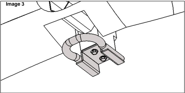
8- Beginning with the driver side, place lower bracket where tow hooks bolts was removed. Use the tow hooks bolts to secure it. Repeat for the opposite side.
