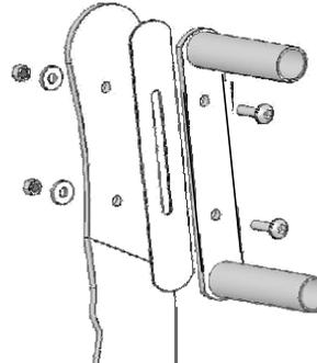
**12-** To install license plate, place the license plate holders at rear edge of the winch tray, use (1) 1/4x1" hex head bolt, (2) 1/4" flat washers, (1) 1/4" lock washers and (1) 1/4" hex nut, for each bracket. Once holders are installed secure license plate with (2) 1/4 x 1" hex head bolt, (4) 1/4" flat washers, (2) 1/4" lock washers and (2) 1/2" hex nuts. Image 9.
