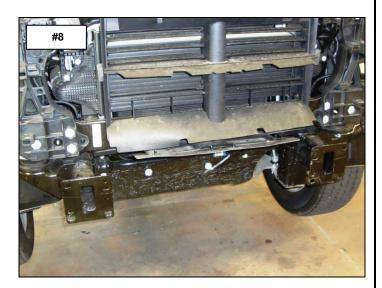
**Step-10** Reinstall the factory grille and radiator dust cover.
