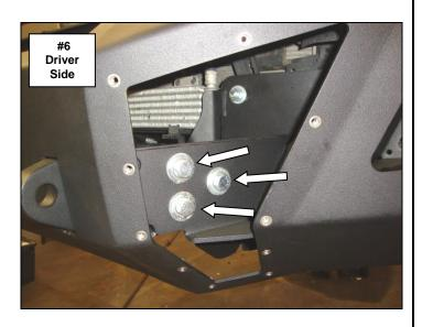
**Step-6** Align the holes and attach each bumper support bracket to the vehicle frame using (2) 3/8" x 1  $\frac{1}{4}$ " hex bolts, (2) 3/8" flat washers, (2) 3/8" lock washers and (2) 3/8" hex nuts, and to the replacement bumper bracket using (1)  $\frac{1}{2}$ " x 1  $\frac{1}{2}$ " hex bolt, (2)  $\frac{1}{2}$ " flat washers, (1)  $\frac{1}{2}$ " lock washer and (1)  $\frac{1}{2}$ " hex nut, (Photo 7).
