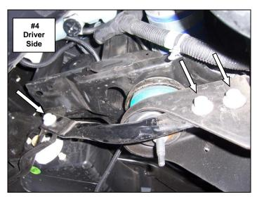
**Step-5** Remove the nut and bolts' securing each of the tow hooks to the frame using an 18mm wrench, socket, and ratchet, (Photo 5). Pull the hooks out from the front and remove from the vehicle.
