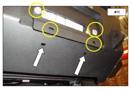
If installing a winch, attach the license plate directly to the (2) obround holes in the lower face of the bumper shell using the supplied 1/4" bolts and nuts, (Photo 11).
