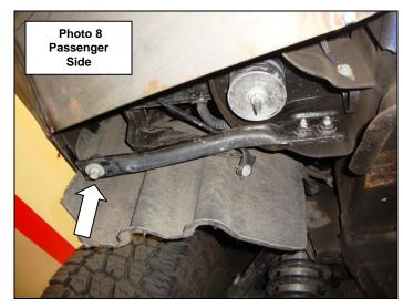
**Step-15** With assistance, adjust and hold the bumper shell visual alignment position, then tighten all factory and supplied nuts and bolts. Note: It may be necessary to loosen the nuts and bolts securing the mounting plate/winch tray and brackets.
