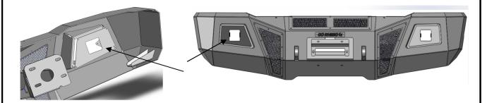
2-. Install the Rigid 4" x 4" D-Series flush mount LED (not included) to the Light Mount Plates using tje nuts and bolts supplied with the lights.
