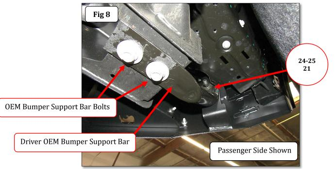
**Step-14** With assistance, adjust and hold the bumper shell visual alignment position, then tighten all factory and supplied nuts and bolts securing the brackets, winch tray and bumper shell. Trim the front fender liners to match the BR5.5 bumper if desired.
