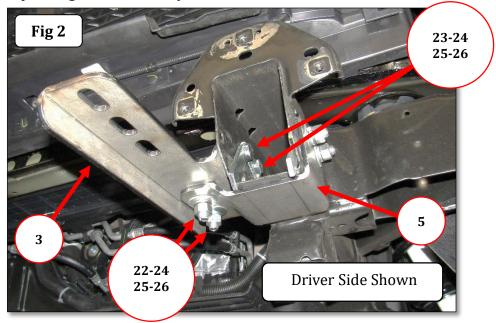
**Step-3** Position the driver side frame bracket up to the end of the frame, align the holes in the frame bracket with the OEM bumper bracket attachment holes in the frame and secure the frame bracket to the frame using (2) of the OEM bumper bracket bolts, (Fig 3). Leave the bolts loose for final adjustment. Repeat to install the passenger side frame bracket.
