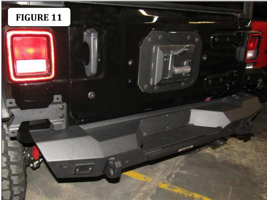
**Step-9** Secure the corner bracket to the weld nuts in the Trailline bumper using (1) 3/8" x 1 1/4" hex bolt, (1) 3/8" lock washer and (1) 3/8" flat washer, (FIGURE 12). Leave the bolt loose for final adjustment. Repeat for the driver side.
