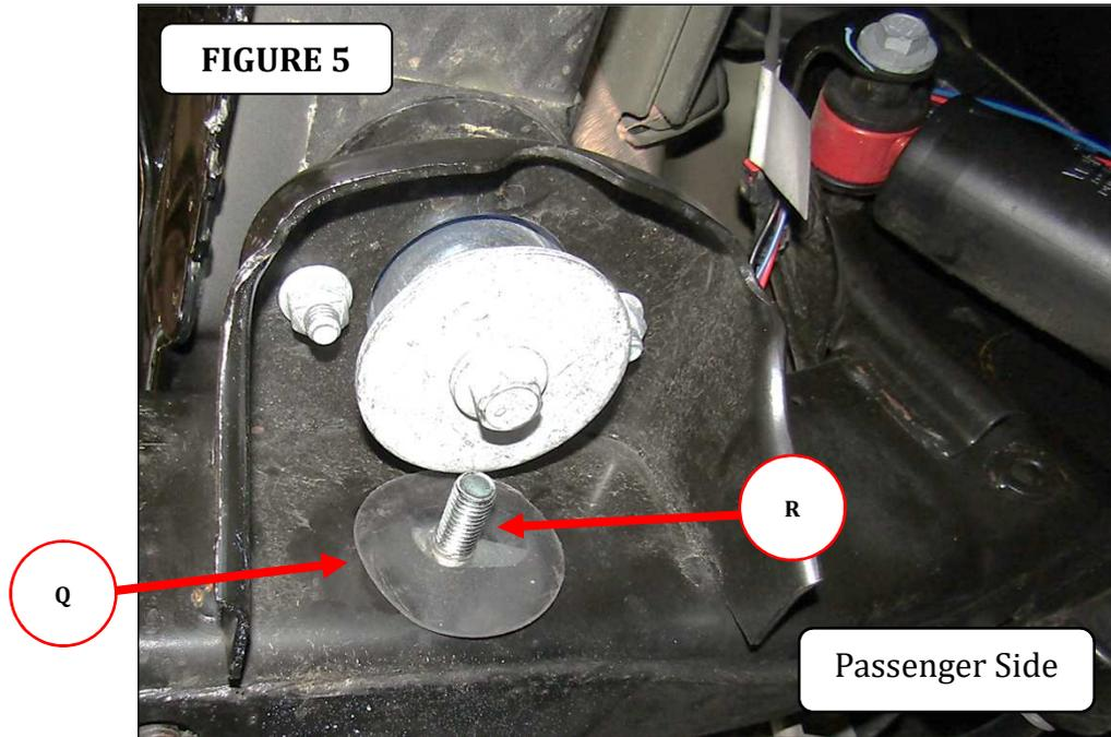
**Step-4** Position the 1/2" double bolt plate inside the passenger side frame rail, so the (2) bolts extend down through the (2) holes in the bottom of the frame rail, (FIGURE 6).
