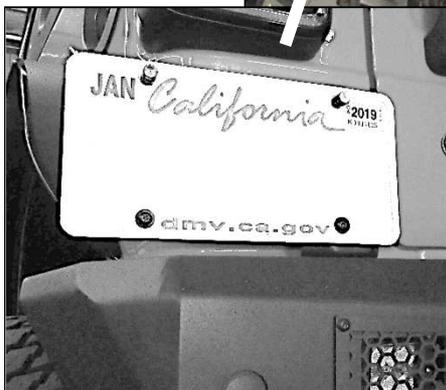
**Step-12** Attach the license plate to the license plate bracket using the supplied  $\frac{1}{4}$ " x  $\frac{3}{4}$ " button head hex drive bolts,  $\frac{1}{4}$ " flat washers,  $\frac{1}{4}$ " lock washers and  $\frac{1}{4}$ " hex nuts.
