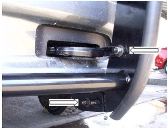
10. Align the grille guard assembly with the front of the vehicle and tighten all assembly and installation nuts and bolts. PHOTO # 9
