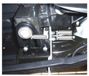
8. To install the auxiliary bracket use the provided template to cut out the bumper's lower cover position the auxiliary bracket through the opening cut out in the lower cover. PHOTO #5 Secure to the tow hook support using a 7/16" x 5" hex bolt, flat and lock washers, and hex nut. Also Attach to the lower bolt of the main bracket. Do not tighten yet repeat the procedure to the opposite side PHOTO #6
