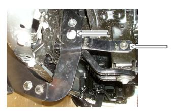
9. Attach the defender with 1/2" x 1 1/2" hex bolts, flat and lock washer and hex nut hand tighten. PHOTO # 7 y 8
