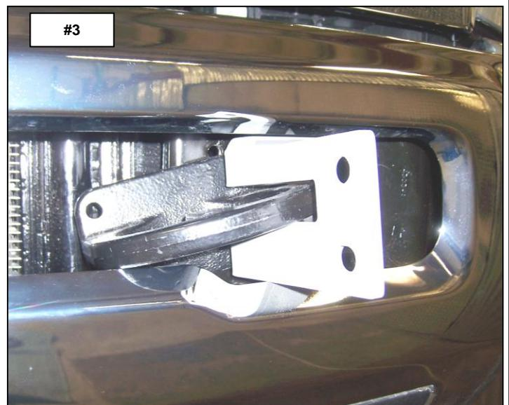
**STEP-3** ATTACH THE TOW HOOK AND THE DRIVER SIDE MAIN BRACKET TO THE VEHICLE USING (2) 3/8" X 2" HEX BOLTS, (4) 3/8" FLAT WASHERS (2) 3/8" LOCK WASHERS AND (2) 3/8" HEX NUTS. **PHOTO #4**
