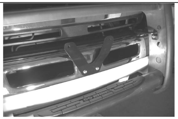
STEP 6. REMOVE THE LICENSE PLATE AND MOUNTING BRACKET FROM THE FRONT BUMPER. ATTACH 1100LP LICENSE PLATE BRACKET TO THE BUMPER USING THE FACTORY SCREWS, AND THE LICENSE PLATE TO THE BRACKET USING THE 1/2" FASTENERS SUPPLIED.
