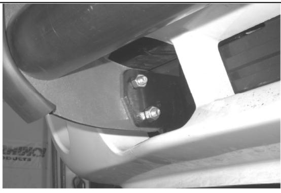
$\textbf{STEP 7.} \ \, \text{ATTACH THE GRILLE GUARD ASSEMBLY TO THE FRAME BRACKETS, AND UPPER BRACKETS USING THE 3/8" X 1" BOLTS, LOCK WASHERS, AND NUTS. ALIGN THE GRILLE GUARD ASSEMBLY WITH THE FRONT OF THE VEHICLE AND TIGHTEN ALL NUTS AND BOLTS.$
