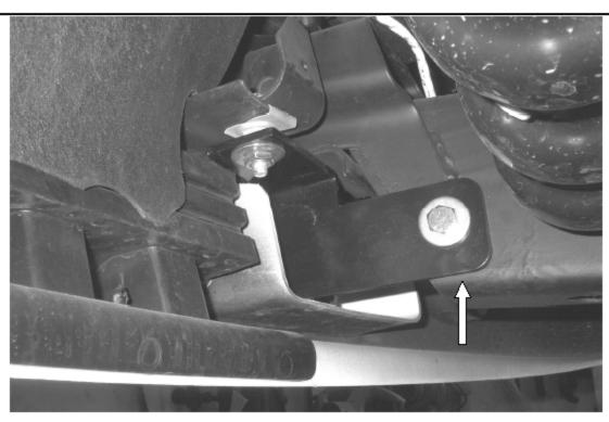
STEP 4. POSITION 1110CP FRAME BRACKET OVER THE SHANK OF THE BUMPER BOLT. LOOSELY ATTACH THE BRACKET TO THE BUMPER BOLT AND FRAME USING THE 12MM HEX NUT, 12MM X 40MM HEX BOLT, AND ½" WASHERS AS SHOWN. NOTE: POSITION THE ¼" THICK WASHER BETWEEN THE BRACKET AND FRAME.
