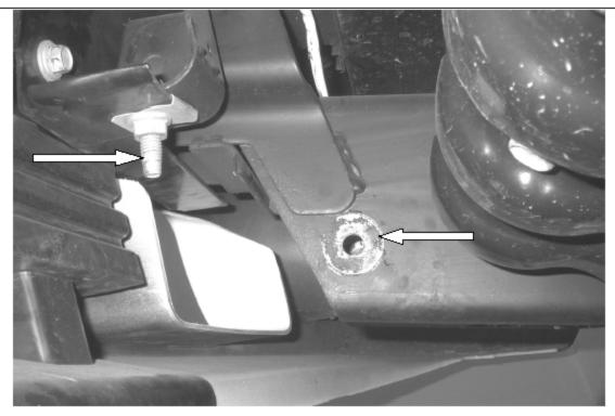
STEP 3. LOCATE THE PASSENGER SIDE BUMPER BOLT AND TOW HOOK MOUNTING BOLTS. REMOVE THE TOW HOOK BOLT FROM THE SIDE OF THE FRAME.
