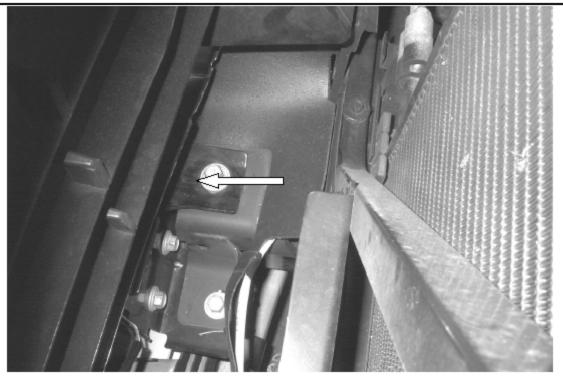
**STEP 1.** BEGINNING WITH THE PASSENGER SIDE, LOCATE AND REMOVE THE UPPER BUMPER BOLT. THE BOLT IS LOCATED BEHIND THE GRILLE NEAR THE TOP OF THE BUMPER. TO ACCESS THE BOLT, REMOVE THE PLASTIC TRIM PANEL ON TOP OF THE GRILLE, UNSNAP THE GRILLE AND REACH DOWN THROUGH THE OPENING.
