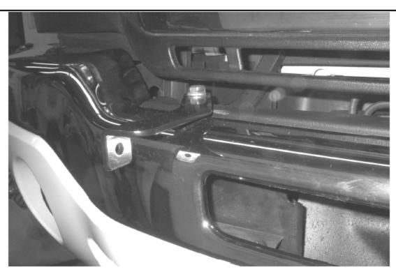
**STEP 2.** POSITION 1100AP UPPER BRACKET THROUGH THE OPENING BETWEEN THE BUMPER AND GRILLE. LOOSELY ATTACH THE BRACKET TO THE BUMPER USING THE 12MM X 120MM BOLT, LOCK WASHER, AND TUBE SPACER.
