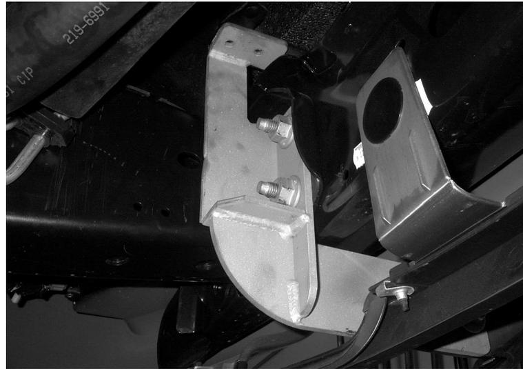
**STEP 4.** INSERT 1122AD UPPER BRACKET THROUGH THE OPENING IN THE GRILLE, AND ATTACH IT TO 1122BD LOWER BRACKET USING THE 5/16" HEX HEAD BOLTS. (FINGER TIGHTEN ONLY).
