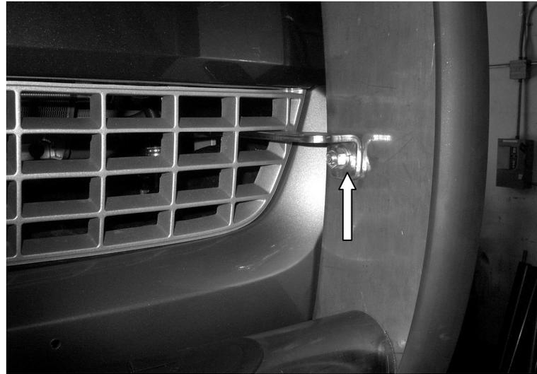
**STEP 8. ALIGN THE GRILLE GUARD ASSEMBLY WITH THE FRONT OF THE VEHICLE AND TIGHTEN ALL MOUNTING NUTS AND BOLTS.**
