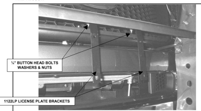
**STEP 9.** IF YOUR STATE LAW REQUIRES A FRONT LICENSE PLATE, ATTACH THE 1122LP BRACKETS, AND LICENSE PLATE TO THE GRILLE GUARD CENTER PLATE USING THE 1/4" BUTTON HEAD BOLTS, WASHERS, AND NUTS.
