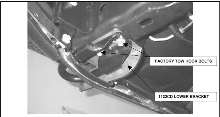
**STEP 3**. POSITION 1123CD LOWER MOUNTING BRACKET BETWEEN THE FRAME AND TOW HOOK. LOOSELY ATTACH THE BRACKET AND TOW HOOK TO THE FRAME USING THE FACTORY BOLTS, AND NUT PLATE. REPEAT THE ABOVE STEPS FOR THE PASSENGER SIDE LOWER MOUNTING BRACKET.
