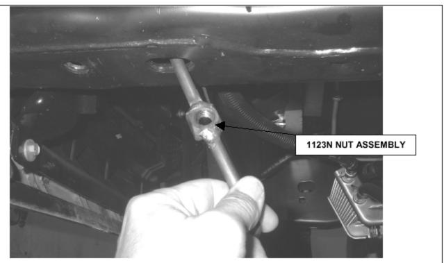
**2 WHEEL DRIVE MODELS**) TO ATTACH THE LOWER MOUNTING BRACKET, POSITION ONE OF THE 1123N NUT ASSEMBLIES UP THROUGH THE LARGER HOLE IN THE BOTTOM OF THE FRAME. ALIGN THE NUTS WITH THE TWO MATCHING HOLES IN THE FRAME, AND ATTACH THE MOUNTING BRACKET USING THE  $\frac{1}{2}$ " X 1  $\frac{1}{2}$ " BOLTS, AND WASHERS SUPPLIED.
