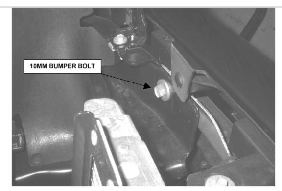
**STEP 4.** OPEN THE HOOD, AND LOCATE THE 10MM BOLT THAT CONNECTS THE BUMPER TO THE BUMPER BRACKET, AND REMOVE THE BOLT.
