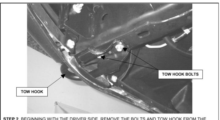
**STEP 2.** BEGINNING WITH THE DRIVER SIDE, REMOVE THE BOLTS AND TOW HOOK FROM THE BOTTOM OF THE FRAME RAIL.
