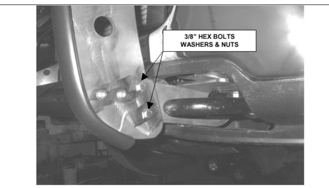
STEP 6. ATTACH THE GRILLE GUARD ASSEMBLY TO THE LOWER MOUNTING BRACKETS USING THE 3/8" X 1 1/4" HEX BOLTS, WASHERS, AND NUTS.
