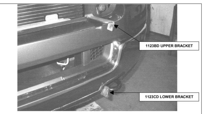
**STEP 5.** ATTACH 1123BD UPPER MOUNTING BRACKET TO THE BUMPER BRACKET USING THE 10MM X 35MM HEX BOLT, AND 3/8" FLAT WASHER. REPEAT THE ABOVE STEPS FOR THE PASSENGER SIDE UPPER MOUNTING BRACKET.
