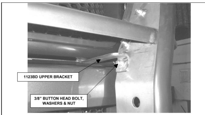
**STEP 7.** ATTACH THE GRILLE GUARD ASSEMBLY TO THE UPPER BRACKETS USING THE 3/8" X 1" BUTTON HEAD BOLTS, WASHERS, AND NUTS.
