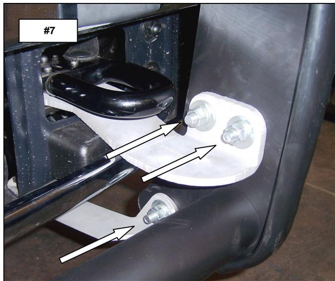
**STEP-9** ALIGN THE GRILLE GUARD ASSEMBLY WITH THE FRONT OF THE VEHICLE AND TIGHTEN ALL NUTS AND BOLTS.
