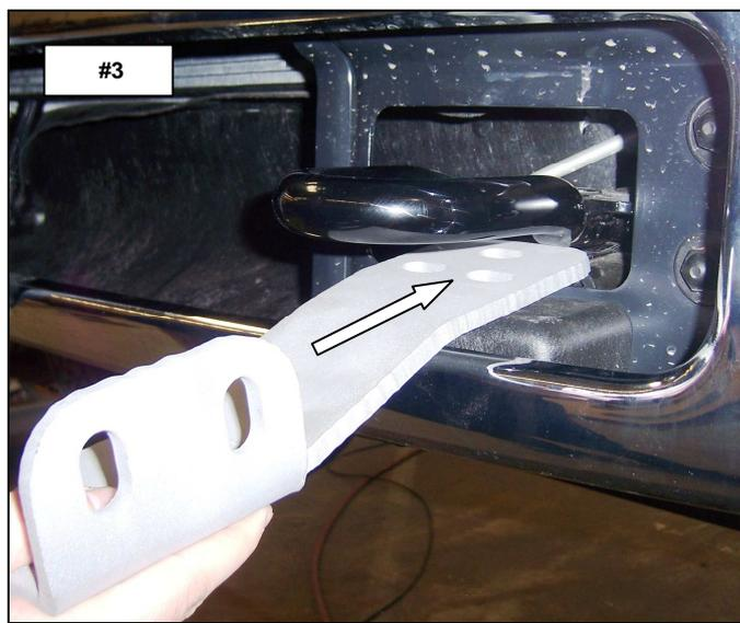
**STEP-5** ATTACH THE UPPER BRACKET AND TOW HOOK TO THE FRAME USING THE FACTORY TOW HOOK BOLTS, DO NOT TIGHTEN. **PHOTO #4**
