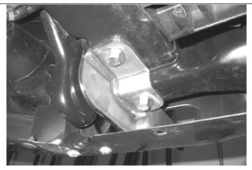
$\tt STEP~2.$  LOOSELY ATTACH 13684D LOWER MOUNTING BRACKET TO THE BOTTOM OF THE FRAME USING THE 12MM BOLTS AND 7/16" WASHERS AS SHOWN.
