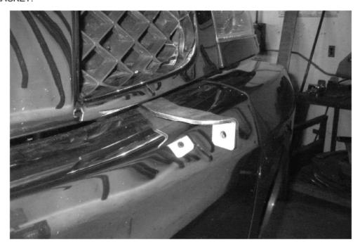
STEP 7. SECURE THE UPPER MOUNTING BRACKETS, AND RE- ATTACH THE GRILLE.
