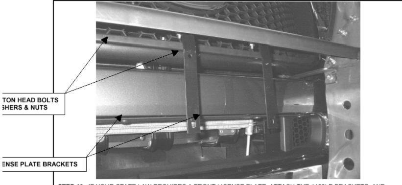
STEP 10. IF YOUR STATE LAW REQUIRES A FRONT LICENSE PLATE, ATTACH THE 1122LP BRACKETS, AND LICENSE PLATE TO THE GRILLE GUARD CENTER PLATE USING THE  $\frac{1}{4}$ ° BUTTON HEAD BOLTS, WASHERS, AND NUTS.
