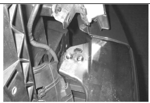
STEP 5. LOCATE AND REMOVE THE (2) BOLTS THAT SECURE THE BUMPER TO THE BUMPER BRACKET.
