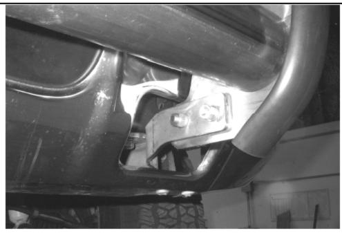
STEP 8. ATTACH THE GRILLE GUARD ASSEMBLY TO THE MOUNTING BRACKETS USING THE 3/8" X 1" HEX BOLTS, WASHERS, AND NUTS.
