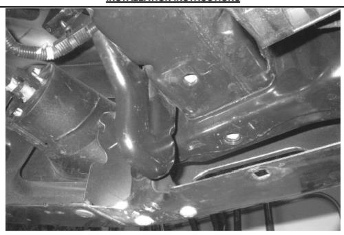
**STEP 1.** BEGINNING WITH THE DRIVER SIDE, IF EQUIPPED, REMOVE THE BOLTS AND TOW HOOK FROM THE BOTTOM OF THE FRAME.
