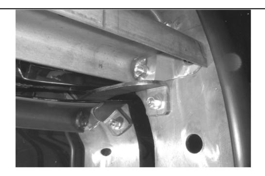
${\bf STEP~9}.$  ALIGN THE GRILLE GUARD ASSEMBLY WITH THE FRONT OF THE VEHICLE AND TIGHTEN ALL MOUNTING NUTS AND BOLTS.
