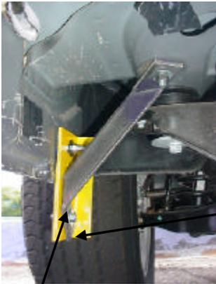
Bracket delantero instalado
