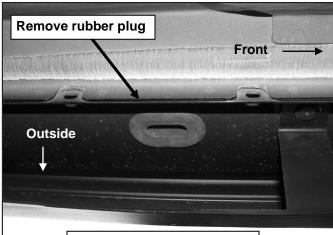
(Fig 1) Driver side pictured from below vehicle
