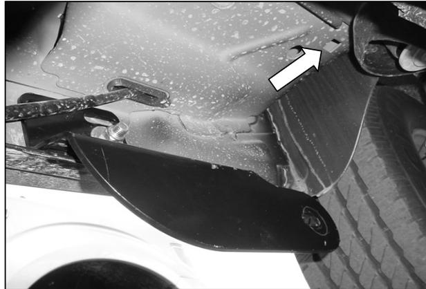
Insert into the square hole steel bar with 5/16" bolt. Front driver's side picture.
