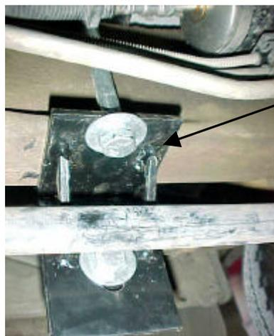
Complemento bracket delantero, lado conductor, vista interior chasis.
