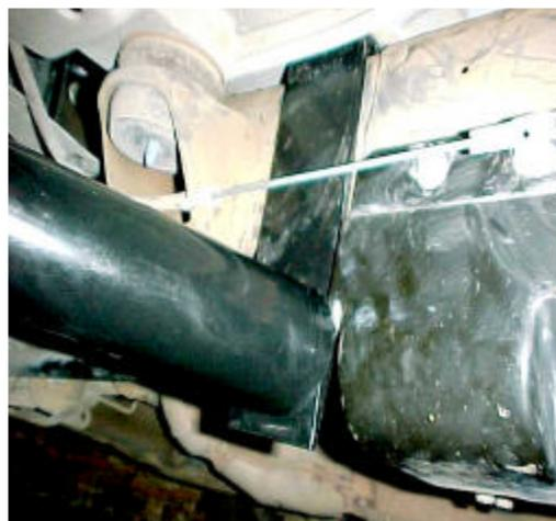
Bracket delantero instalado, lado conductor
