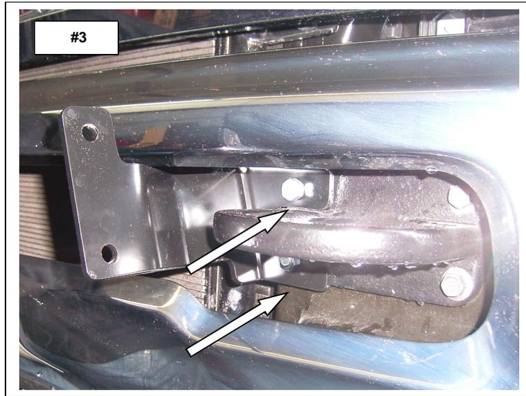
**STEP-3** POSITION THE RHINO CHARGER BAR MOUNTING TABS BETWEEN THE DRIVER AND PASSENGER SIDE BRACKETS AND ATTACH THE TABS TO THE BRACKETS USING (2) 3/8" X 1" HEX BOLTS, FLAT WASHERS, LOCK WASHERS AND HEX NUTS. **PHOTO #4**
