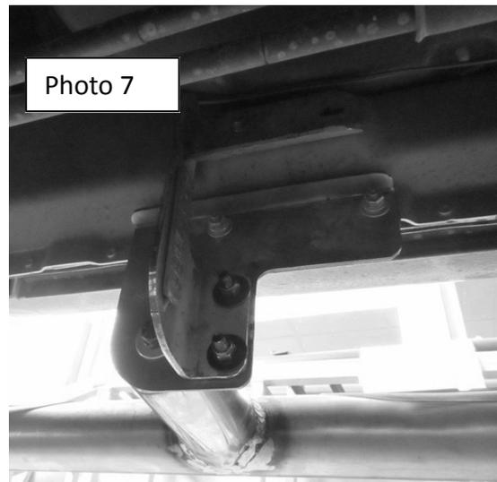
6. Attach the wheel to wheel to the center bracket using (1) 5/16" x 1" hex bolt Black P., (1) 5/16" flat washer Black P. and (1) 5/16" spring lock washer Black P. Leave the nuts loose for final adjustment. **(Photo 8)**
