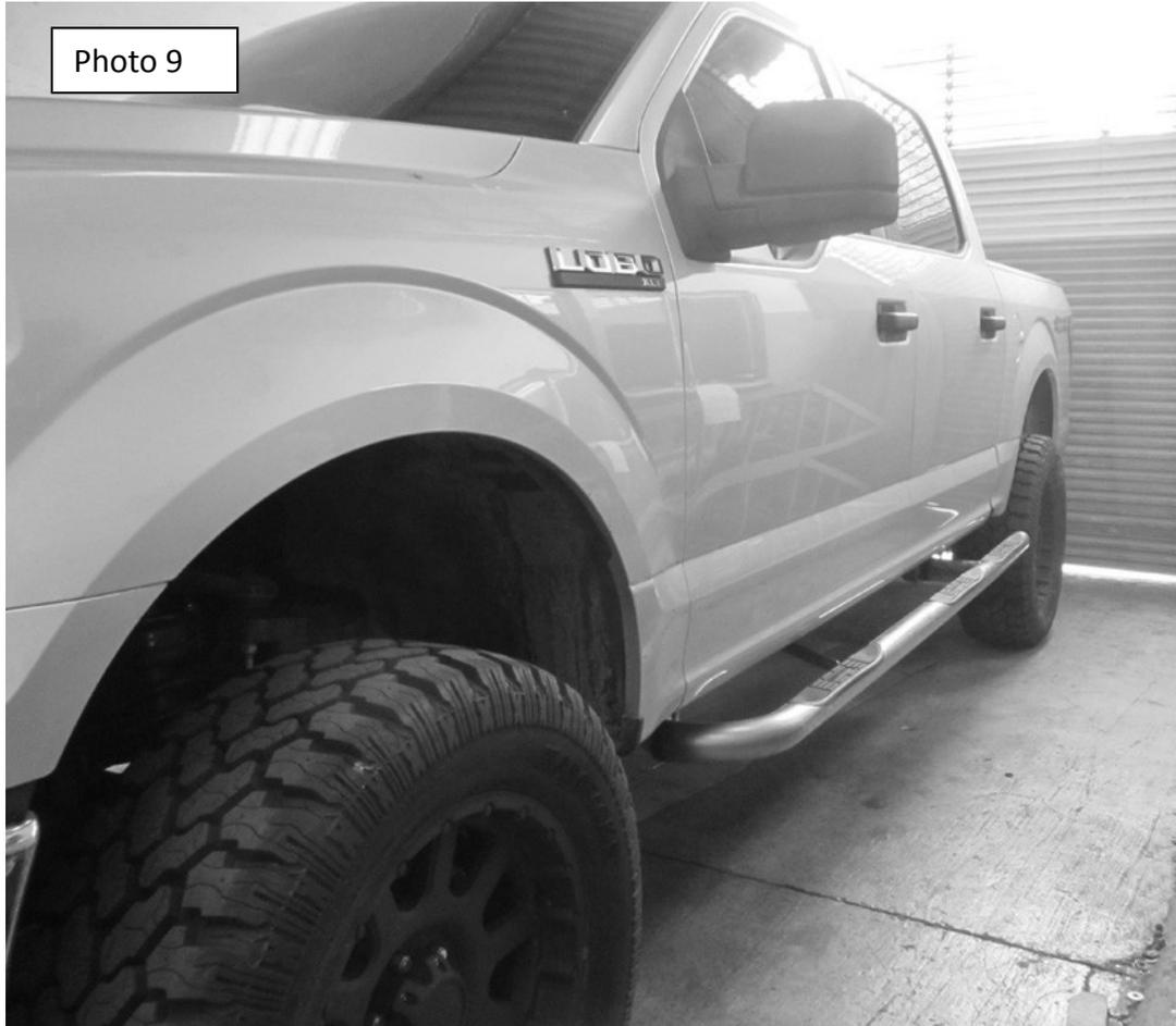
8. Repeat the above process to install the passenger side brackets and side bar.
