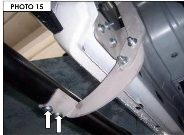
14. Make any final adjustments to the alignment of the sidebar and tighten all bolts, starting with the brackets.
