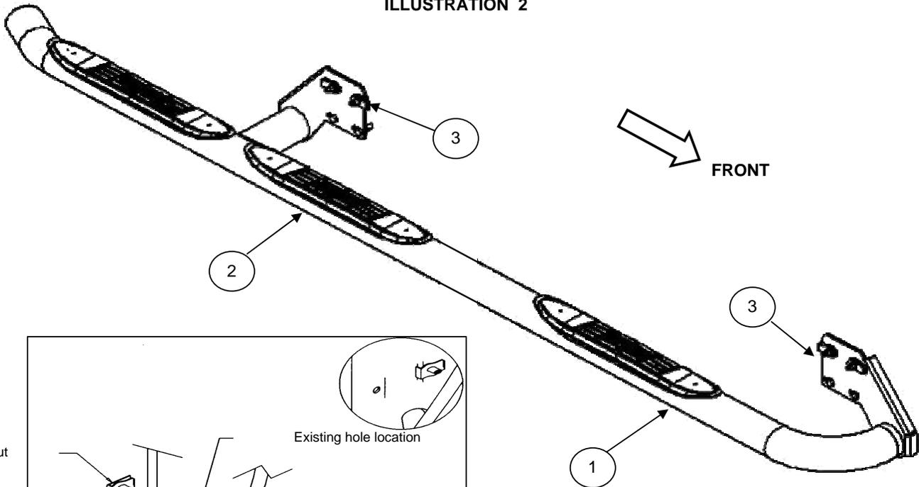
Position in Rocker panel to install brackets.
