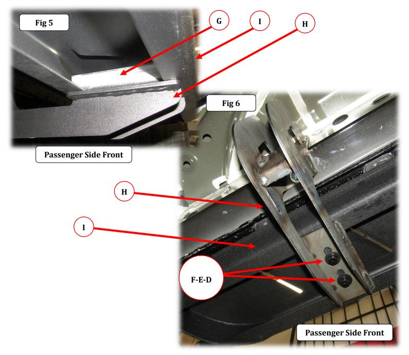
**Step-5** Align the running board with the vehicle and tighten all supplied nuts and bolts securing the running board and bracket assembly. Repeat to install the passenger running board.
