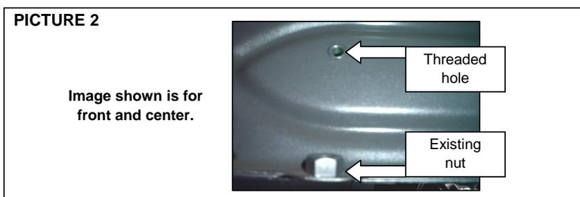
**Step-2** Locate in the center and rear in the rocker panel of the vehicle the hole and insert a M8 clip nut. **SEE PICTURE 3 & 4 & 5.** Place the bracket and attach with: M8 hex head bolt, M8 flat and lock washers, M8 hex nut (zinc plated), according to the **ILLUSTRATION 2.** Leave loose. Repeat for the opposite side.
