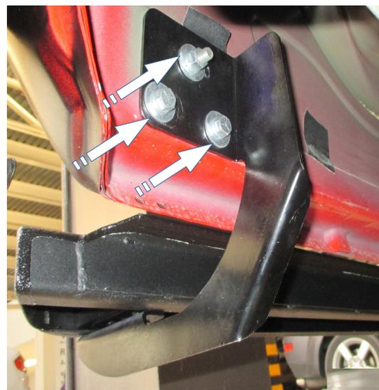
7. Place the sidebar on top of the mounting brackets. Position (3) of the U-brackets (included with the side step) inside the sidebar body, and align the U-brackets with the mounting brackets. Attach the side step and U-brackets to each mounting brackets using (2) 5/16" Hex head bolts, (2) 5/16" flat washers and (2) 5/16" lock washers. **ILLUSTRATION 3.**
