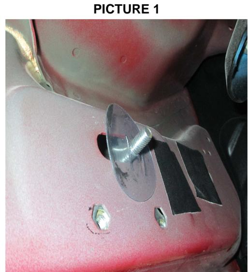
5. Place the front and middle bracket and attach to the bolt of the plate that was placed in the panel of the vehicle with: 3/8" flat and lock washers, 3/8" hex nut secure.
