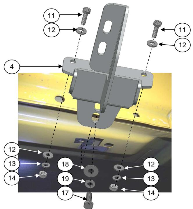
**STEP 4.** LOCATE THE HOLES IN THE BODY PINCH MOLD AND REMOVE THE TAPE COVERING THE THREADED HOLE IN THE UNDER SIDE OF THE BODY AT THE REAR OF THE VEHICLE. **PHOTO #5**
