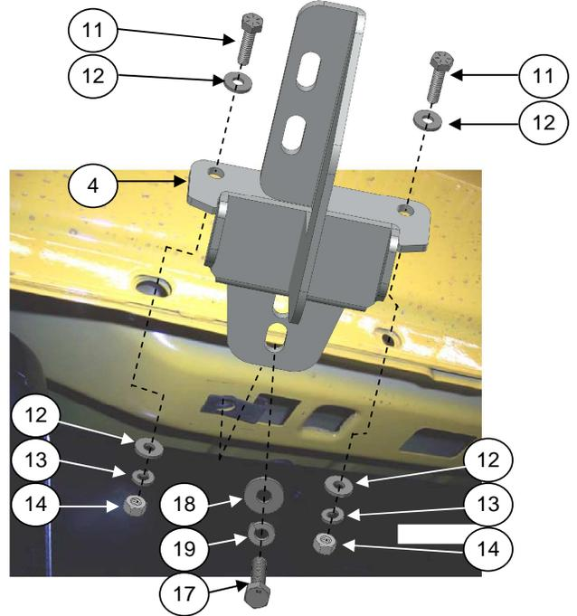
**STEP 3.** REPEAT THE ABOVE PROCEDURE TO INSTALL (1) MIDDLE MOUNTING BRACKETS AT THE CENTER POSITION. DO NOT TIGHTEN. **PHOTO #3 & PHOTO #4**
