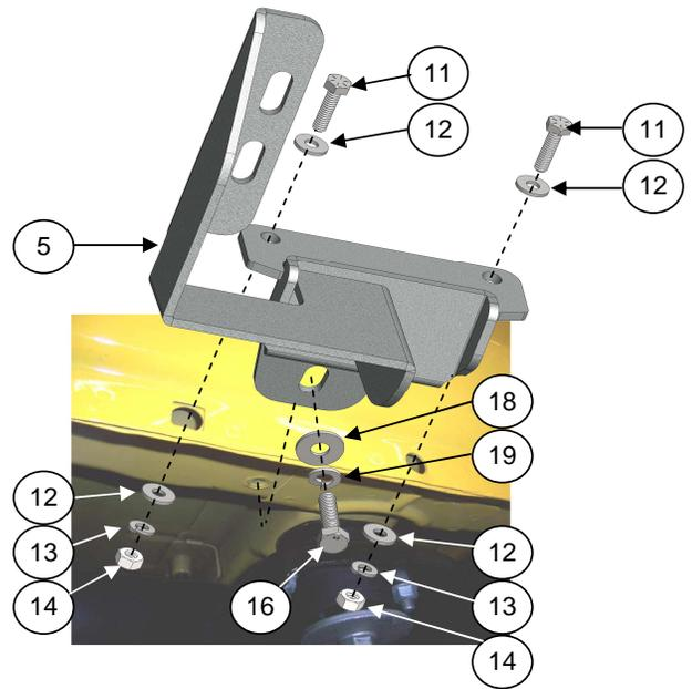
**STEP 6.** PLACE THE U BRACKET INSIDE RB10 SIDE STEP, PLACE THE RB10 SIDE STEP ON BRACKETS AND ATTACH WITH: 5/16" HEX HEAD BOLT, 5/16" FLAT AND LOCK WASHER (BLACK PLATED), BY EACH BRACKET. **PHOTO #7**
