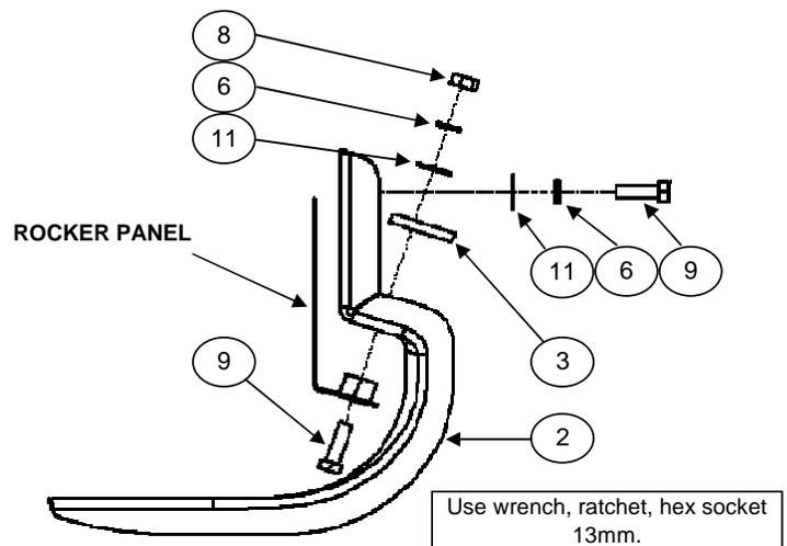
5. For **EXTENDED CAB** models, locate in the rear in the rocker panel of the vehicle the hole and insert a M8 clip nut. **SEE PICTURE 2**. Place the bracket and attach according to the **ILLUSTRATION 2**. Repeat for the opposite side.
