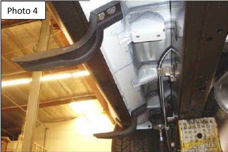
8. Attach the passenger Step Bar to the mounting brackets using the supplied M8 hex head bolts, flat washers and lock washers.
