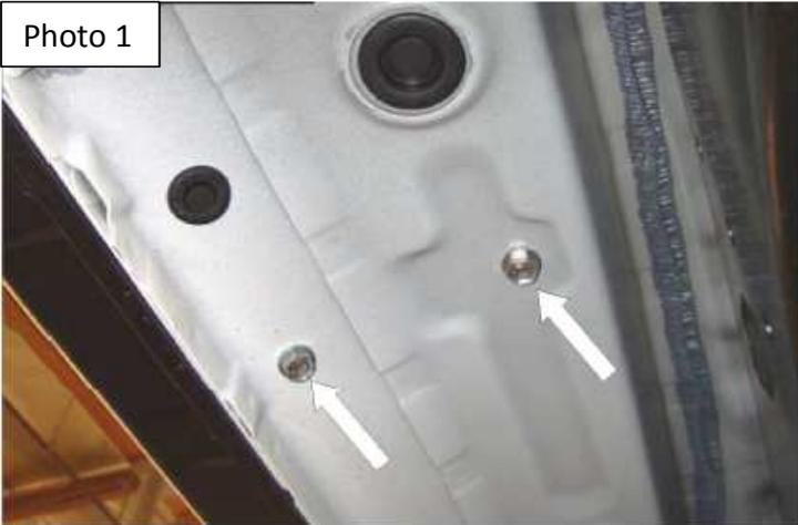
5. Remove & discard the factory bolts from the center and rear bracket mounting locations. **(Photo 2)**
