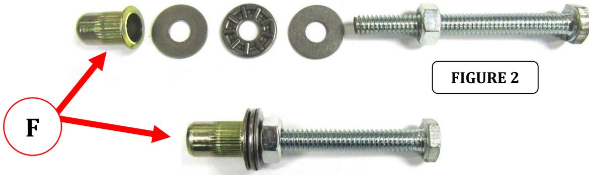
**Step-5** Place the rivet-nut with the attached tool components into the enlarged hole in the body structure. Use a 7/16" wrench to hold the nut, and tighten the bolt using a 7/16" wrench or socket and ratchet. Continue tightening the bolt until the rivet-nut is fully compressed and no longer spins then remove the tool components, (FIGURE 3).
