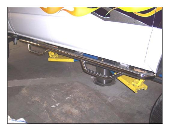
**Step 6.** Align sidestep with the body and then tighten all mounting bracket and sidestep nuts and bolts. **Step 7.** Repeat the above installation steps to install the driver side mounting brackets and sidestep.
