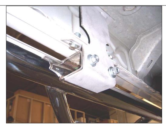
**Step 5.** Position the passenger sidestep up to the mounting brackets and loosely attach it to the brackets using the 3/8" x 1" hex bolts, flat washers, lock washers and nuts.
