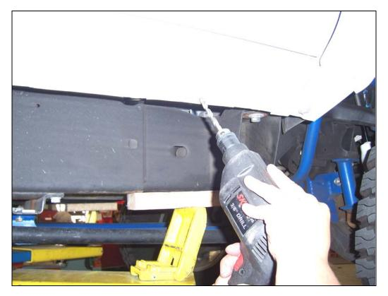
**Step 3.** Confirm the measurements, center punch and drill 3/8" holes through the body pinch mold. Repeat the above procedure for the driver side.
