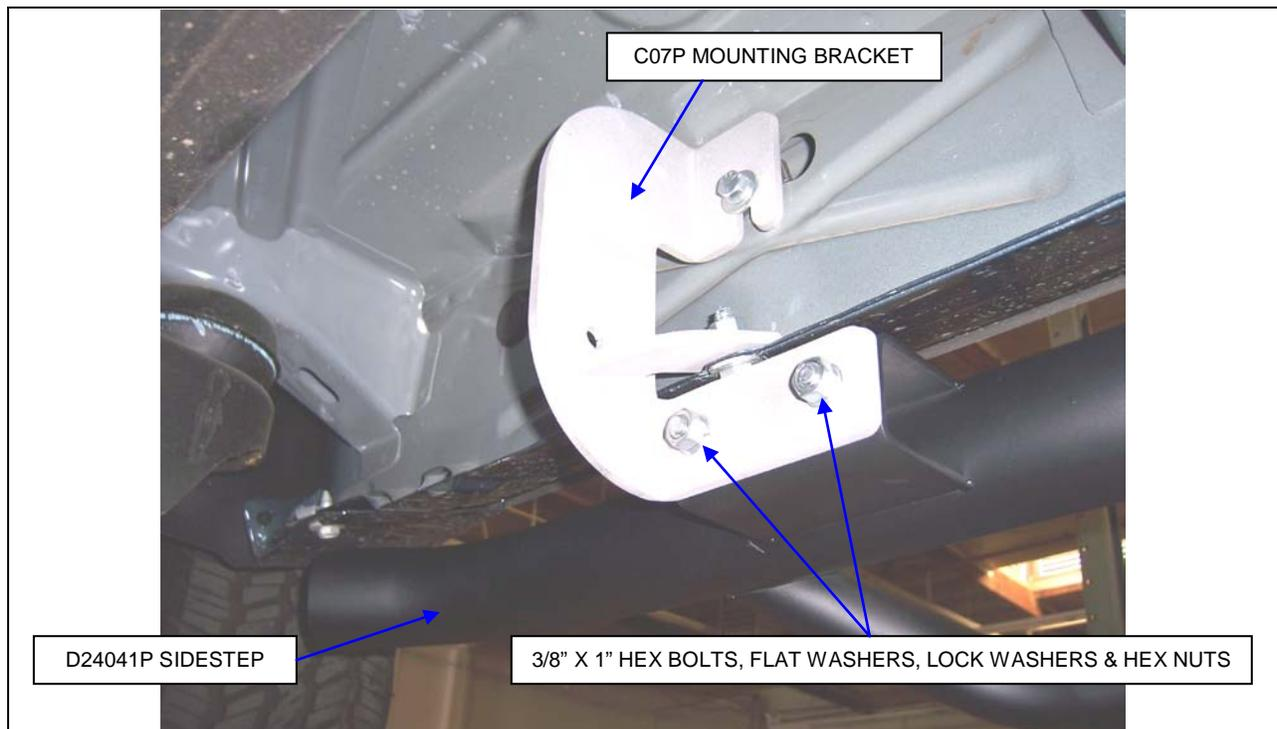
**STEP 6.** Position D24041P passenger sidestep up to the vehicle and loosely attach it to the mounting brackets using the 3/8" x 1" hex bolts, flat washers, lock washers and hex nuts.
