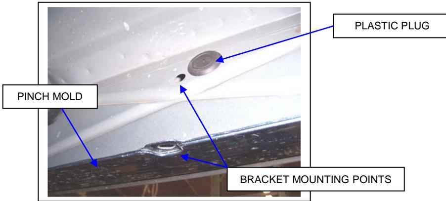
**STEP 3.** Remove the plastic plug from the rocker panel and install (1) 5/16" U-NUT as shown.
