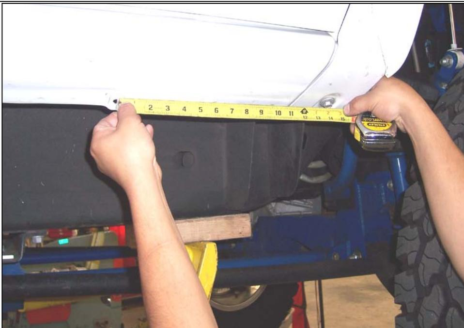
**STEP 2.** This installation uses three mounting brackets per side. Begin by installing the passenger side front mounting bracket. Measure rearward from the front fender bolt approximately 14" and Locate the single hole in the body pinch mold and the two holes in the rocker panel.
