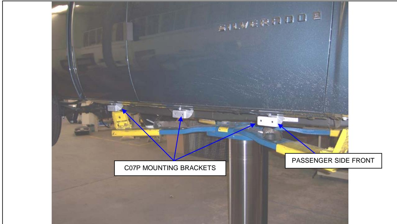
**STEP 5.** Locate the holes in the body for the center and rear mounting brackets. Measure rearward from the front fender bolt 37 3/4" for the center and 67" for the rear bracket. Repeat steps 3 & 4 to install the center and rear brackets.
