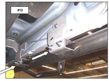
Step-8 Align the side step with the vehicle and tighten all nuts and bolts.
