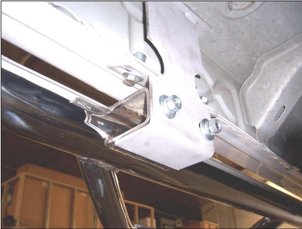
**Step 5.** Position the passenger sidestep up to the mounting brackets and loosely attach it to the brackets using the 3/8" x 1" hex bolts, flat washers, lock washers and nuts.
