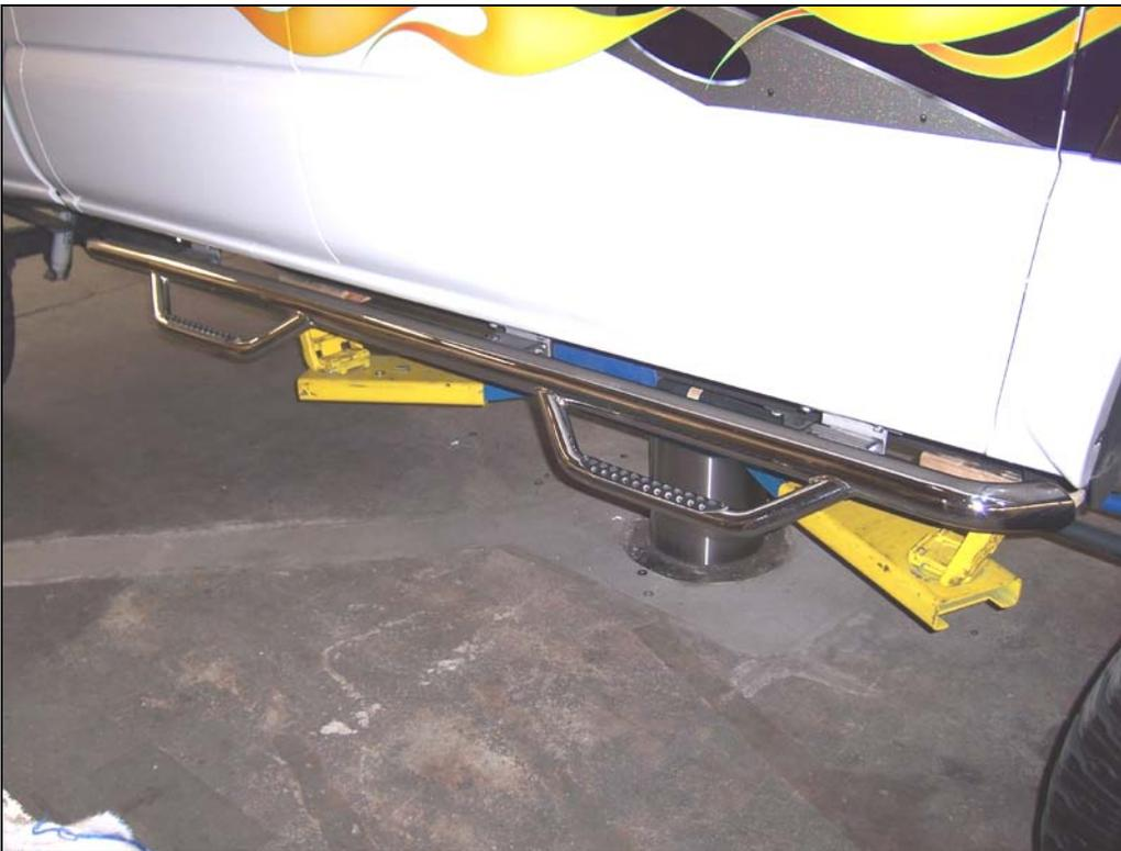
**Step 6.** Align sidestep with the body and then tighten all mounting bracket and sidestep nuts and bolts.
